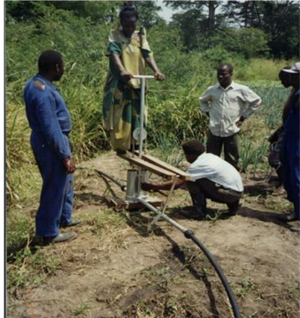
Figure 5-11 Treadle pump: Money maker model (left); NARO-AEATREC Model (right)
