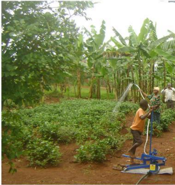
Figure 5-11 Treadle pump: Money maker model (left); NARO-AEATREC Model (right)
