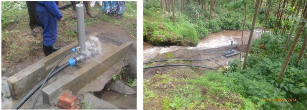
Figure 5-14 AEATREC-NARO low drive-head hydraulic ram pump model
